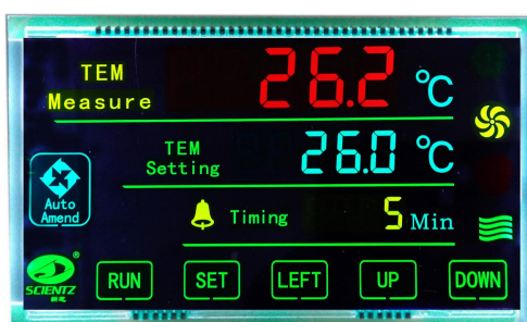
P3—1 Single point temperature and time setting
